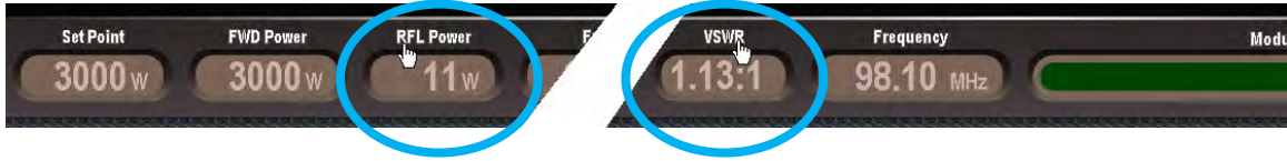
Figure 34 – VSWR or Reflected Power Display
