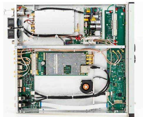
Below is the inside of the 30W translator / OCDR system showing PSU, PRO-TV board and amplifier
