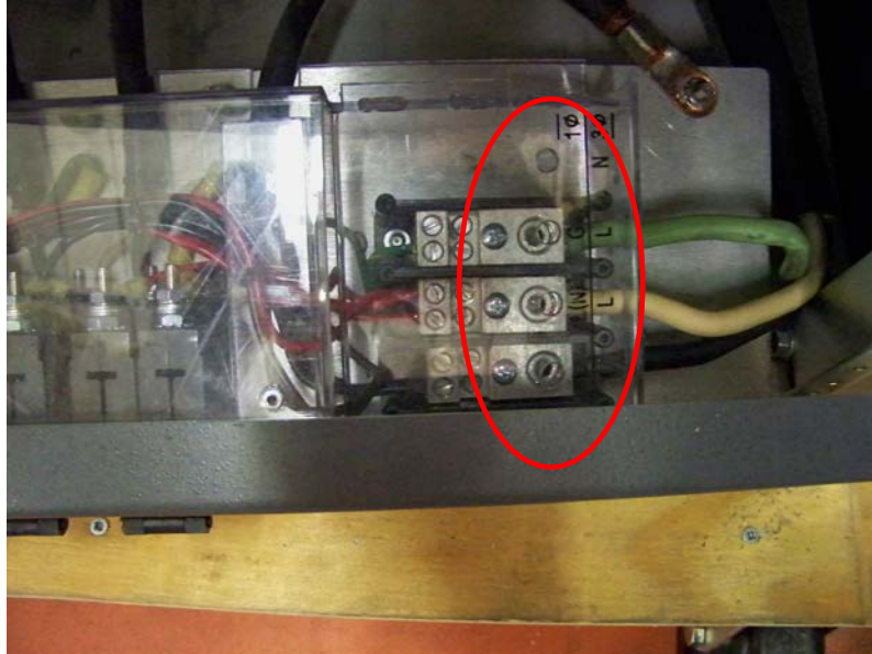
Figure 8. Remove input AC wiring.
