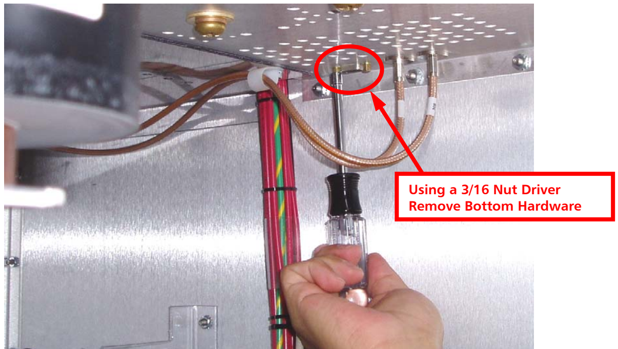
Figure 17 – Feedthru Connector Hardware Removal
