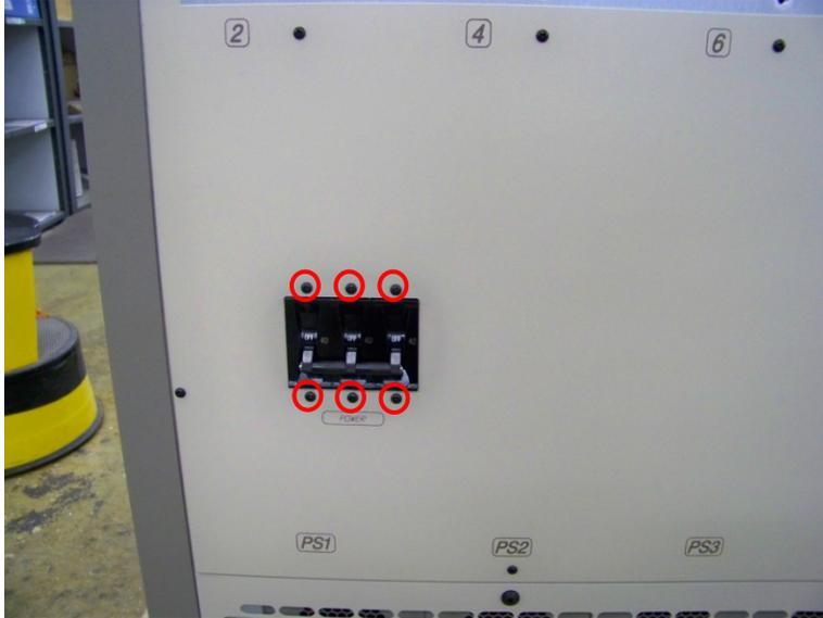
The PA modules do not have to be removed to perform this procedure. Remove the front cabinet panel by removing the 25 Philips head screws. Set screws aside for reinstallation later.
