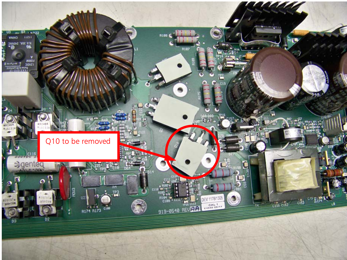
Figure 11 – Heat sink removed from board
