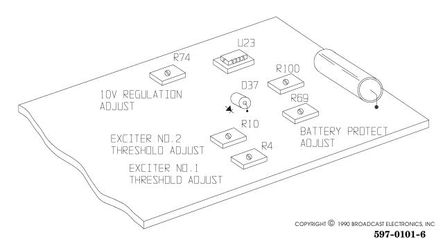
FIGURE 5-1. FW-30 CONTROL LOGIC CIRCUIT BOARD ADJUSTMENTS
