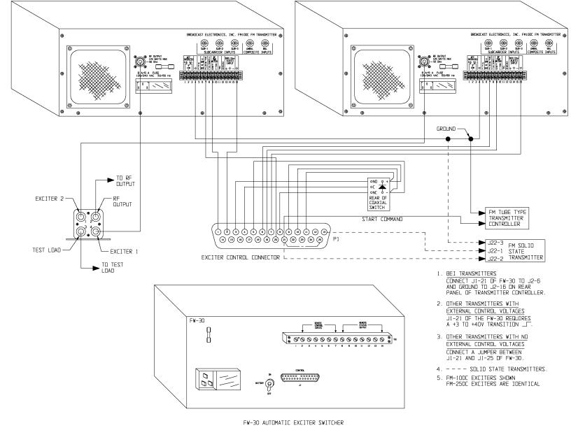
FW-30 INTERFACING - FM-100C/FM-250C SYSTEMS FIGURE 2-1. FW-30 INTERFACING (SHEET 2 OF 2)
