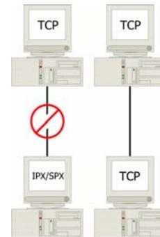
The IP (Internet Protocol) suite is the closest thing that the computer world has to a universal language. It is also routable, meaning it's easier to connect multiple segments over a wide area network. The two most common transport protocols, or languages, in the suite are TCP (Transport Control Protocol) and UDP (User Datagram Protocol.)
