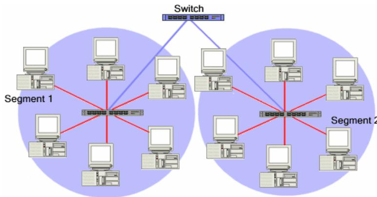
A switch is a network device that separates multiple segments on a network, but is smart enough to know if a particular packet needs to be sent to the other side.
