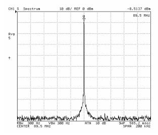
**Figure 6:**Carrier at 89.5MHz, 0dB reference, ∼10dB attenuation added
