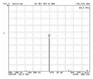
**Figure 3:**Carrier at 89.5MHz, 0dB reference, 49dB notch on carrier
