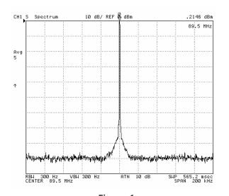
Figure 1: Carrier at 89.5 MHz, 0dB reference, no notch
