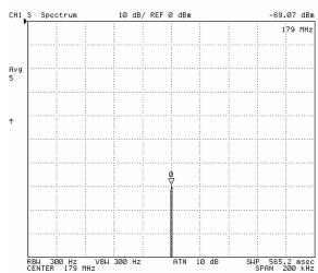
Figure 2: 2<sup>nd</sup> harmonic at 179 MHz, with carrier at 0dB reference, no notch
