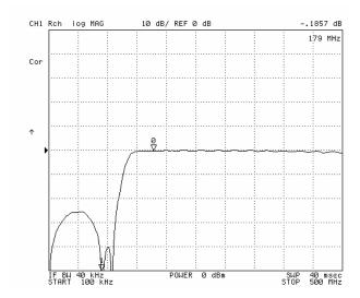
**Figure 5**: Notch Filter Performance, ~50dB attenuation at 89.5MHz, 0.2dB attenuation at 179MHz
