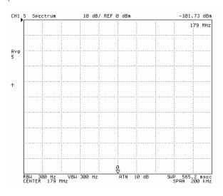
**Figure 4:**2<sup>nd</sup> harmonic at 179MHz, with carrier at 0dB reference, notch on carrier
