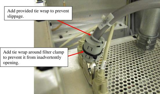
Figure 2. Filter clamp attached to control cable.
