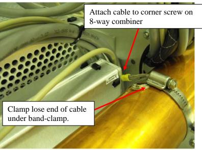
Figure 3. RFI Eliminator ground connection on FM-20S/1405.
