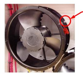
Use a 5/16" Nut Driver or Open End Wrench and remove the fan mounting hardware ( 3 places per fan)
