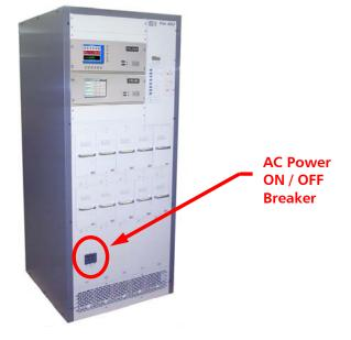
Figure 14 – Transmitter ON / OFF Breaker Location
