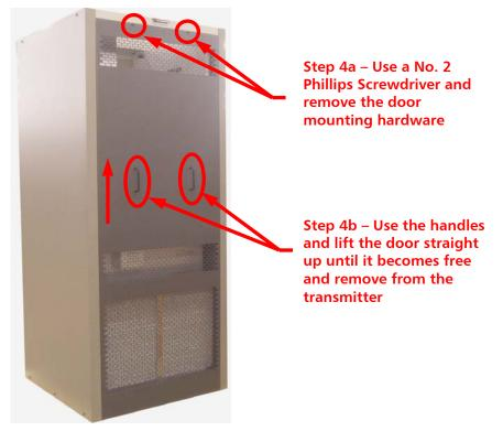
Figure 3 – Remove Outer Rear Panel
