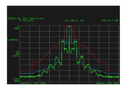
Figure 4 - Misaligned AM Transmitter
