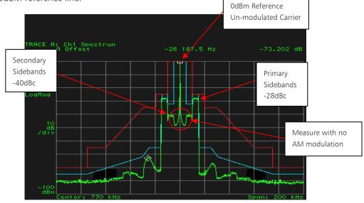
Figure 3 - 0dBm reference (Aligned AM IBOC Transmitter)
