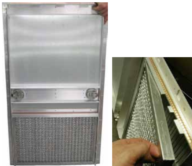
Figure 160 – STX HP Air Filter
