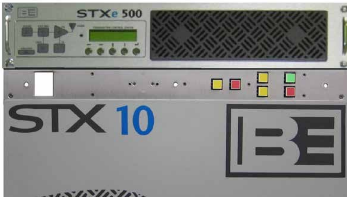
Figure 198 – STX HP Front with 1RU Silkscreened Panel Removed
