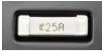
Figure 106 – 25A Final Amplifier Fuse
