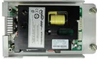
Figure 168 – 24/12+VDC Power Supply
