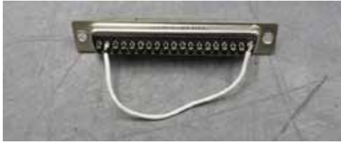
Figure 16 – Exciter GPIO Connector for Stand-Alone
