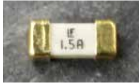
Figure 102 – 1.5A Low Voltage Fuse
