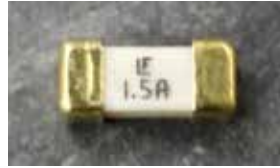
Figure 104 – 1.5A Driver Amplifier Fuse
