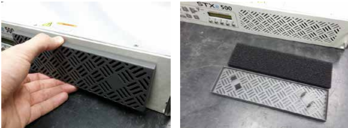
Figure 59 – STXe 500 Air Filter Removal
