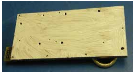
Figure 121 – Pallet with Thermal Compound
