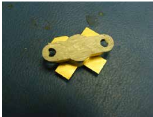
Figure 111 – Driver with Thermal Compound Applied
